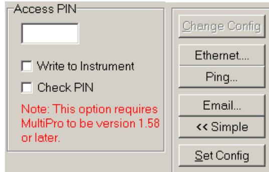
7. Enter a unique 4-digit PIN in the input box under Access PIN and click on "Write to Instrument".
