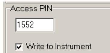
8. Click "Set Config" to tell the dock to upload the PIN setting to the instruments. The software will automatically show the Security Login screen a second time and prompt you for your user name and password. Once a valid User ID and Password have been entered, "PIN Lock Writing Enabled" will be shown in the dock configuration window. The dock is now ready to upload the PIN to the instruments.
