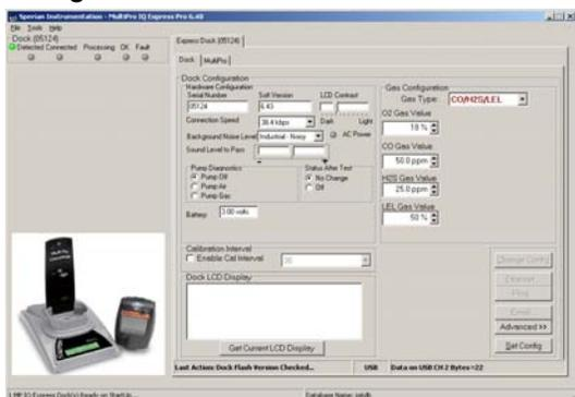
To change the configuration of the MultiPro IQ Express Dock that is displayed, click on the “Change Config” button at the lower right of the screen. Once the dock configuration is uploaded, the “Set Config” button will be enabled. Once changes are made, click on the “Set Config” button to save the new settings.
