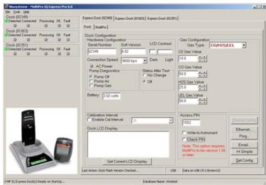
5. Click "Advanced" in the row of buttons on the lower right. The software will automatically show the Security Login screen and prompt you for your user name and password. If the "Advanced" button is not shown, click on "Change Config" first to access it.
