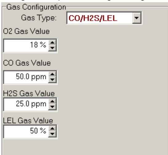
Note: The gas values shown in the gas configuration screen are the values that will be used in calibrating the MultiPro instruments that interface with the dock regardless of the MultiPro’s own built-in calibration gas settings.
