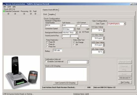
The screen is divided into right and left sides. The left side gives the status of the docks that are currently installed and
