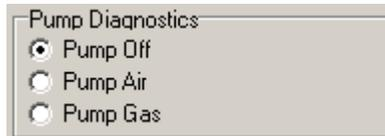
Click “Pump Gas” to draw span calibration gas through the right gas port at the back of the dock. Click “Pump Air” to draw the fresh air sample through the left gas input port.
