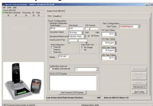
**Note:** If the “Change Config” button is enabled, press it before making any changes to the settings.
