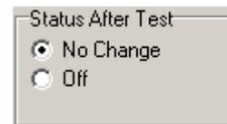
If “Status After Test” is set to Off, the MultiPro will automatically be turned off by the dock once the instrument has been processed.
