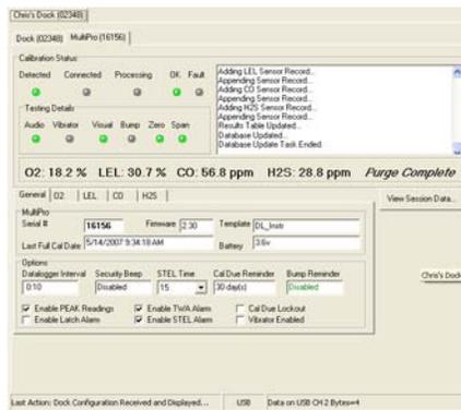
The output box is updated as the instrument is detected, connected, and processed. When faults occur, the details of the fault will be shown and a red fault light will be shown. Below, a span calibration failure is the cause of the fault.
