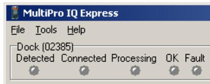
When a detector is placed in the dock, the indicator will change to reflect the new status. Status changes are also shown on the dock's LCD.
