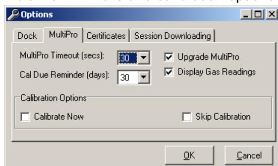
The Timeout setting controls the amount of time that needs to pass after connection between the dock and the PC is lost before the instrument will reset itself. Options are in 5-second increments from 5 to 30 seconds. To change the setting, click on the arrow to the right of the timeout setting to access the list and select the new setting.
