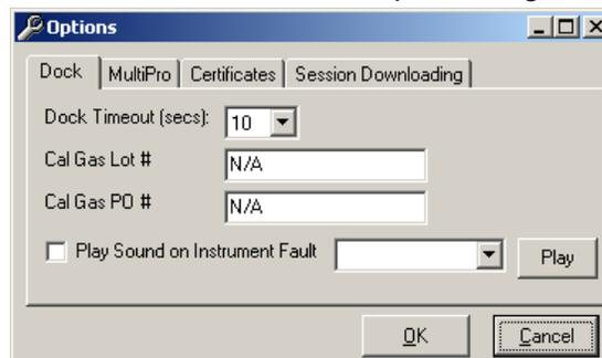
The Dock Timeout Setting controls the amount of time that needs to pass after connection between the dock and the PC is lost before the system will notify you that the connection has been lost.
