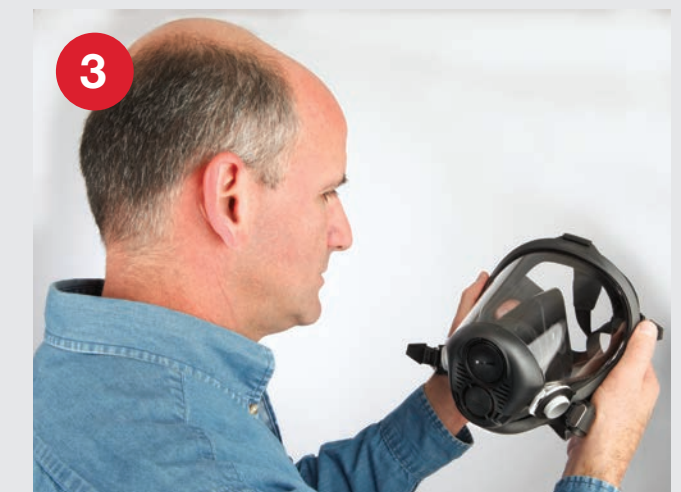
3 Check the lens to make sure it is not cracked or shows signs of crazing.
