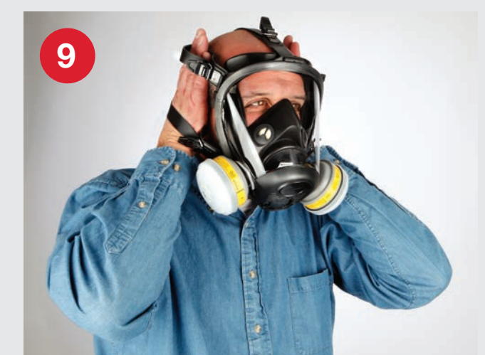
9 Place the headstraps on your head, pushing any hair backward and away from your forehead. Continue pulling the straps over your head until the harness is centered toward the back of your head. DO NOT TIGHTEN AT THIS TIME.
