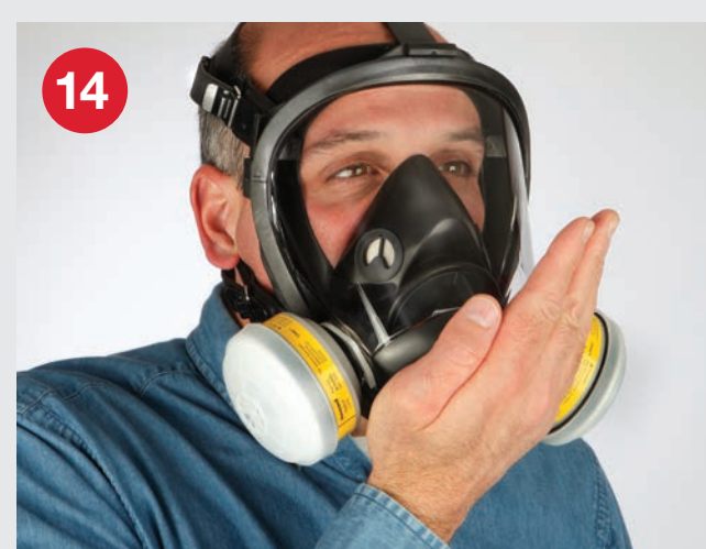
14 Positive Pressure Seal Check: Place the palm of your hand over the exhalation valve so it is completely sealed and exhale gently. If you have a good seal, the facepiece will be pushed away from your face very slightly.
