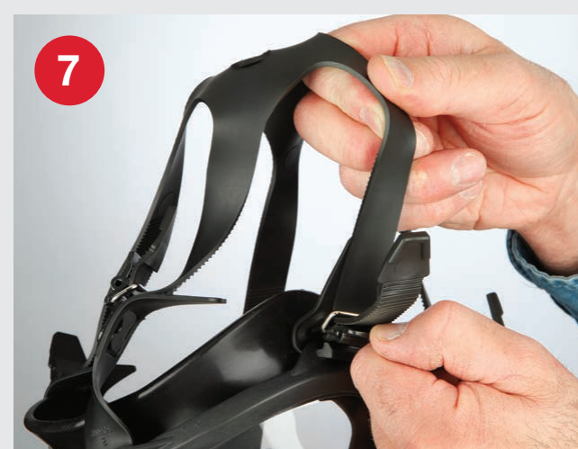
7 Adjust the respirator head straps to their full outward position.
