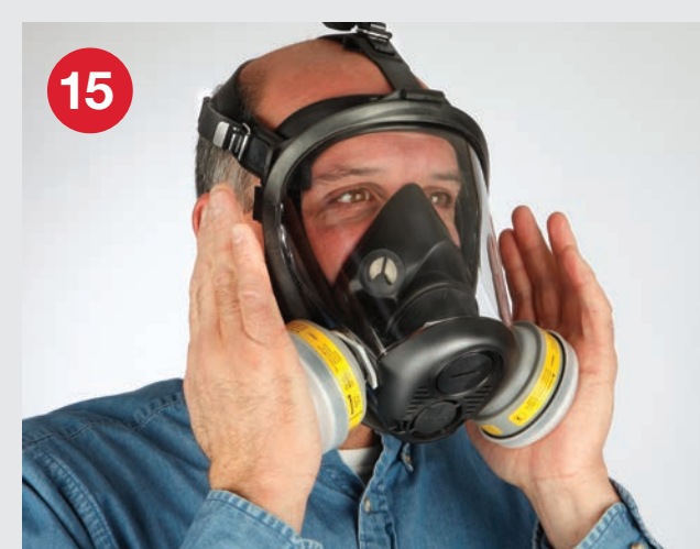
15 Negative Pressure Seal Check: Place the palm of each hand over the two cartridges or filters so they are completely sealed and inhale. Hold your breath for 5 seconds. If you have a good seal the facepiece will be pulled inward toward your face.
