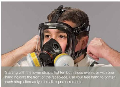
Starting with the lower straps, tighten both sides evenly, or with one hand holding the front of the facepiece, use your free hand to tighten each strap alternately in small, equal increments.
