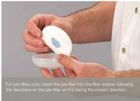
For pre-filters only: Insert the pre-filter into the filter retainer following the directions on the pre-filter so it is facing the correct direction.
