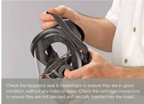
Check the facepiece seal & headstraps to ensure they are in good condition, without any holes or tears. Check the cartridge connectors to ensure they are not cracked and are fully inserted into the mask.
