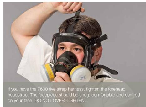
If you have the 7600 five strap harness, tighten the forehead headstrap. The facepiece should be snug, comfortable and centred on your face. DO NOT OVER TIGHTEN.
